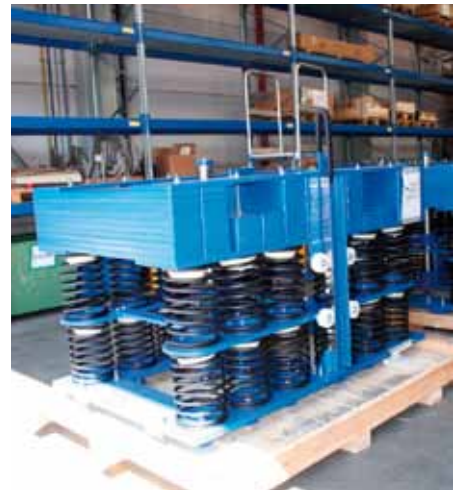
MAURER mass dampers produced in Munich
