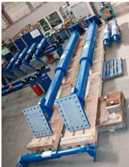
MAURER hydraulic dampers produced in Munich
