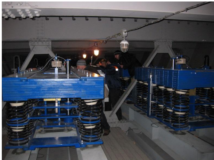
Fig. 21 – Frequency control tests at the Universität der Bundeswehr München with the controlledTMD of the Volgograd Bridge and final functional check of the controlledTMDs installed in the Volgograd Bridge
