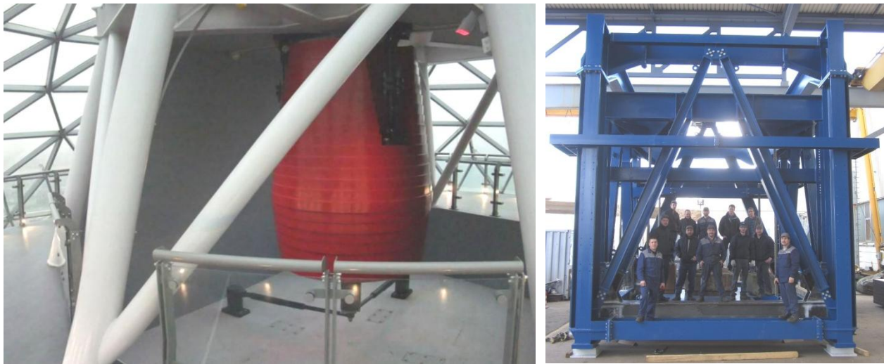
Fig. 3 – standardTMD constructed in pendulum form and foldedTMD in workshop in Munich
