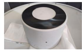
Unusual insight: a puck, the centrepiece of a SIP<sup>®</sup>-Bearing. The photo was taken during the overhaul of a prototype bearing following testing. *Photo: MAURER*
