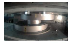
Prototype testing of the SIP® bearing at EUCENTRE Pavia.
