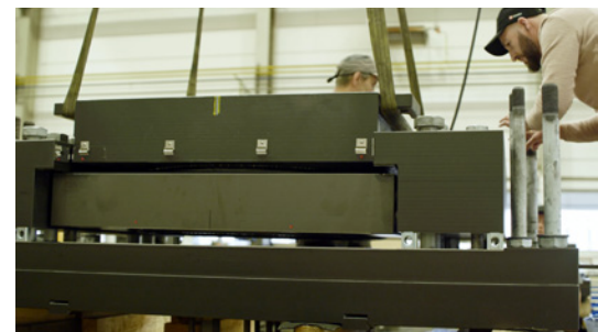
In the production, the centrepiece, which is the actual bearing, is inserted.
