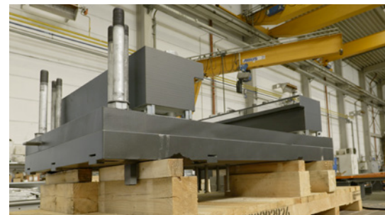
In the production at MAURER: Clearly visible the external clamps with sliding plate (shining), which prevent the bearings from opening in the case of uplift forces.
