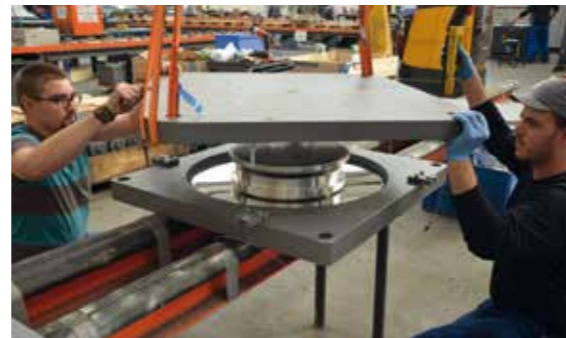
Assembly of SIP®-Adaptive
